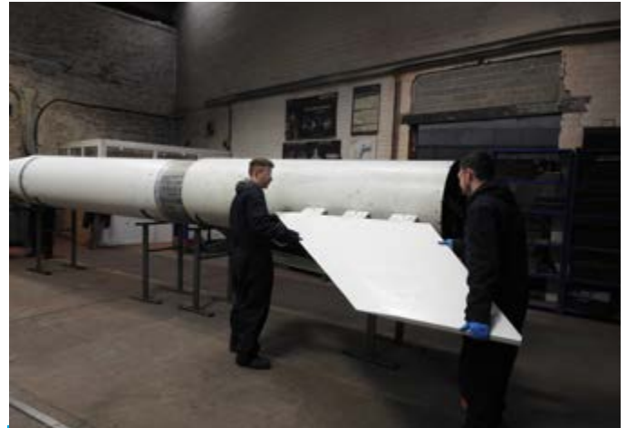
WEC apprentices assembling the Skybolt 2 rocket
